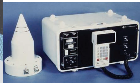
A TI4100 GPS receiver developed and built by Texas Instruments in the early 1980s, the first field-deployable GPS receiver on the market. Calgary-based Nortech Surveys ordered the first four commercial units produced in 1981 and used them to successfully conduct surveys around the world for the ocean-exploration and energy industries until the late 1980s.
