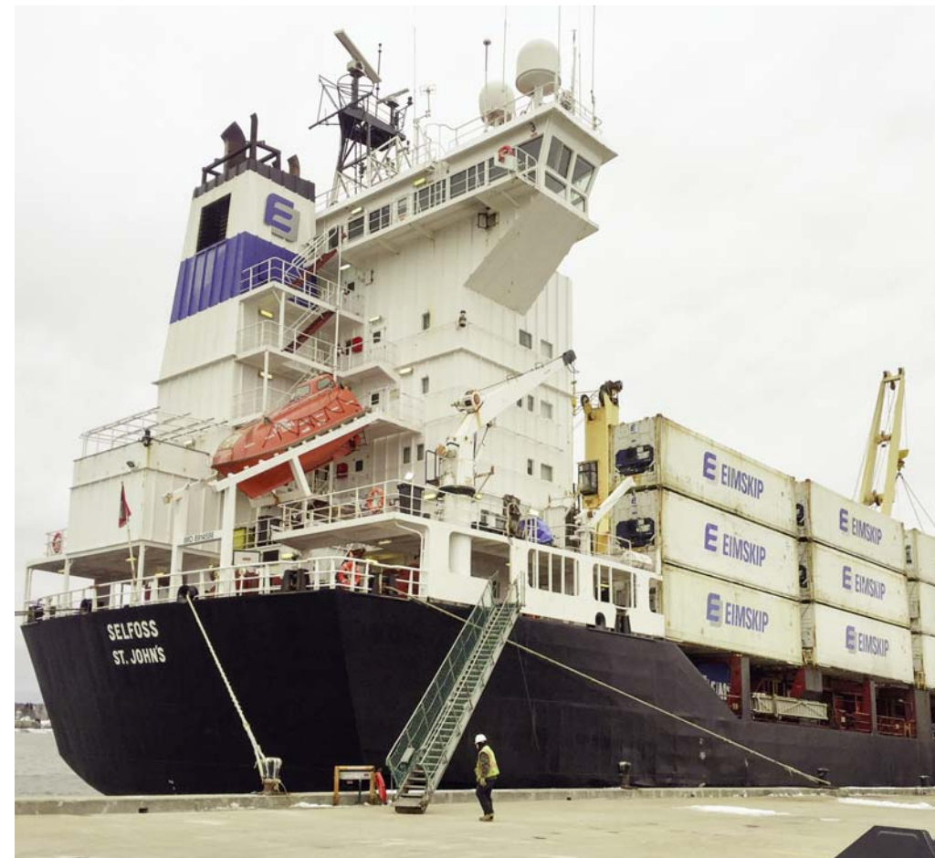
The bridge on the container ship Selfoss is seven stories up. The living spaces for the crew are housed in the tower below the bridge.
