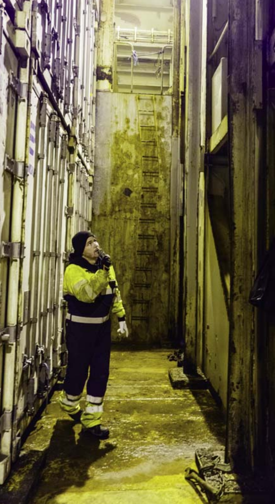
Every six hours a crew member checks each refrigerated container and the ties holding them down. The containers are tracked using a digital recorder, which logs temperature and other data.
