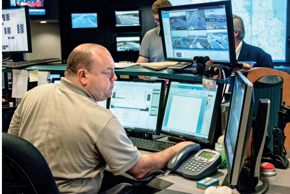
At its data center in Smyrna, DelDOT can monitor traffic conditions and use computers to control nearly all of the state's 1,000 traffic signals in an effort to keep vehicles moving.
