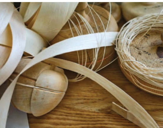
Frey splits and cuts the strips into various widths and thicknesses. Some are braided into fine strands, unique to his basketry. He weaves his baskets over wooden molds.
