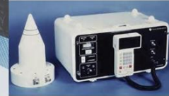
A T14100 GPS receiver developed and built by Texas Instruments in the early 1980s, the first field-deployable GPS receiver on the market. Calgary-based Nortech Surveys ordered the first four commercial units produced in 1981 and used them to successfully conduct surveys around the world for the ocean exploration and energy industries until the late 1980s.
